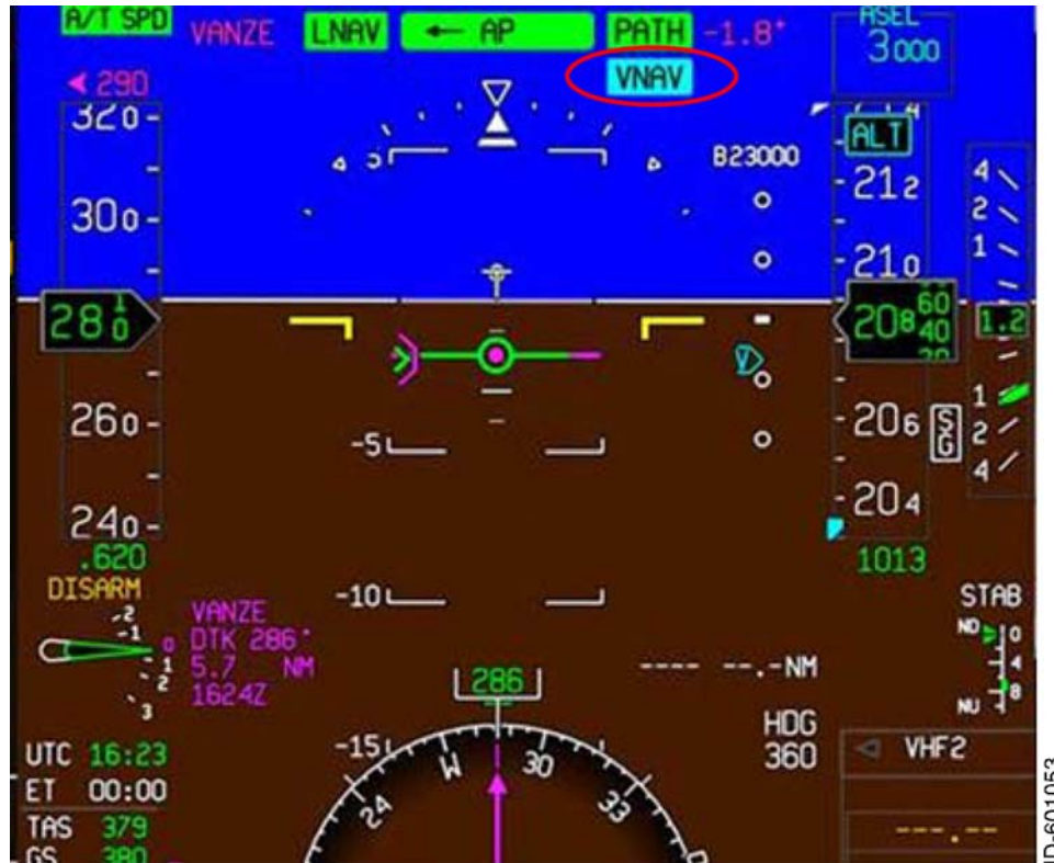
Figure 2. (Sheet 1 of 1) VNAV is Armed and Unable to Capture VNAV PATH while Sequencing VANZE
