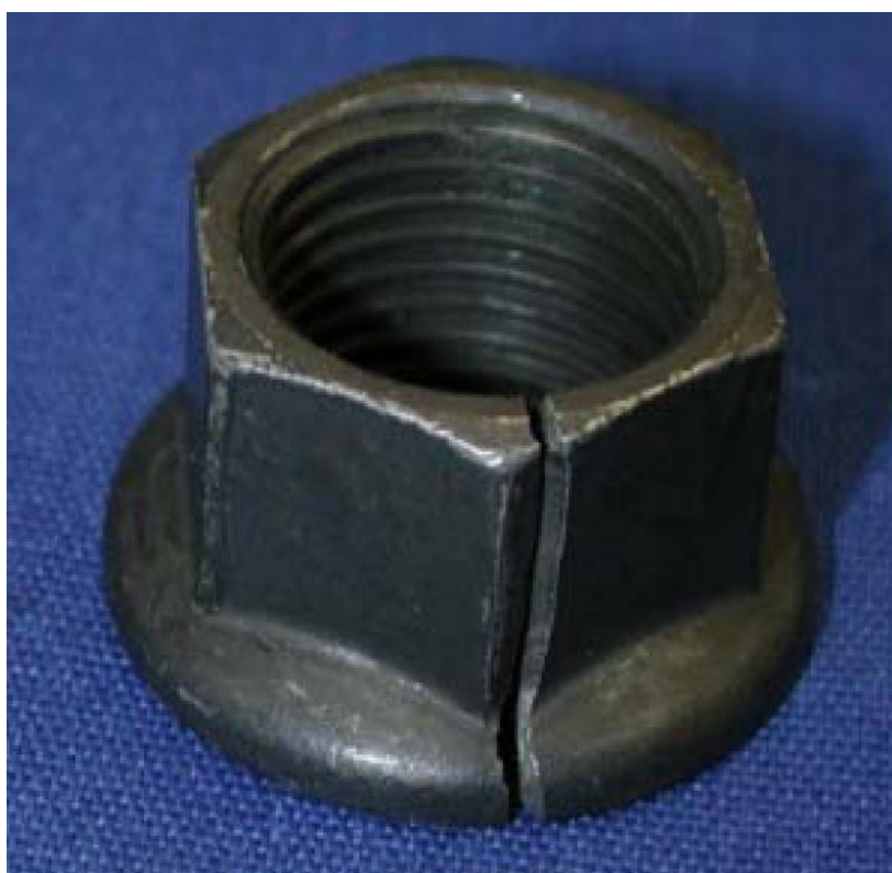
Figure 3: Example of longitudinal crack.
